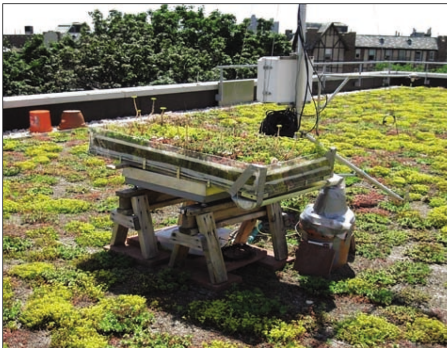
Working with a graduate student at Drexel University, Gaffin and his team have successfully installed and are running an innovative new method for measuring water retention on the upper roof. They have built a scale model of the roof (shown above) and are literally weighing the scale model every five minutes so they can see how much rain is absorbed and how quickly.
